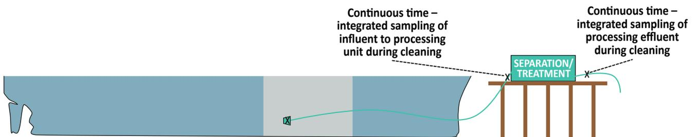
Figure 2: Schematic arrangement of sampling.
