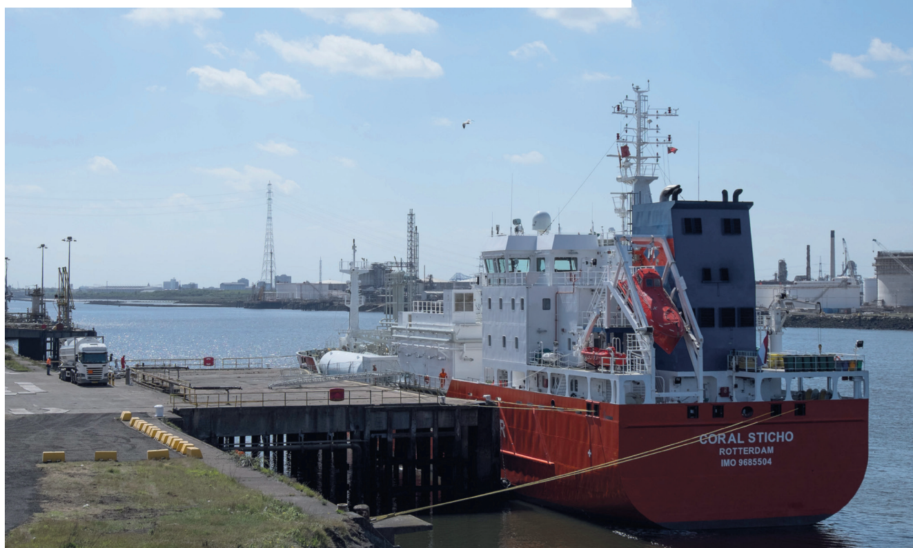
Shell organised the summer 2015 Teesside LNG bunkering of Anthony Veder's gas-powered ethylene carrier Coral Sticho, prior to the commissioning of a dedicated bunkering facility in the port
