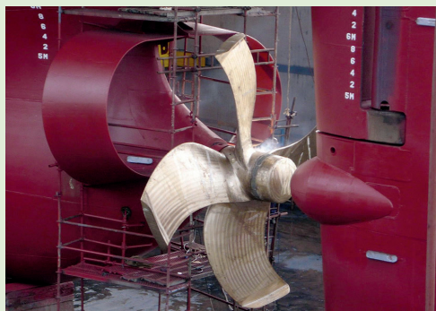
Image of pre-flow duct, high-efficiency, contracted and loaded tip (CLT) propeller and rudder bulb
